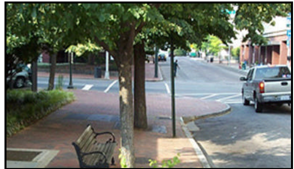
This "choker" at the Medical College of Virginia helps to slow, but not impede traffic flow.
